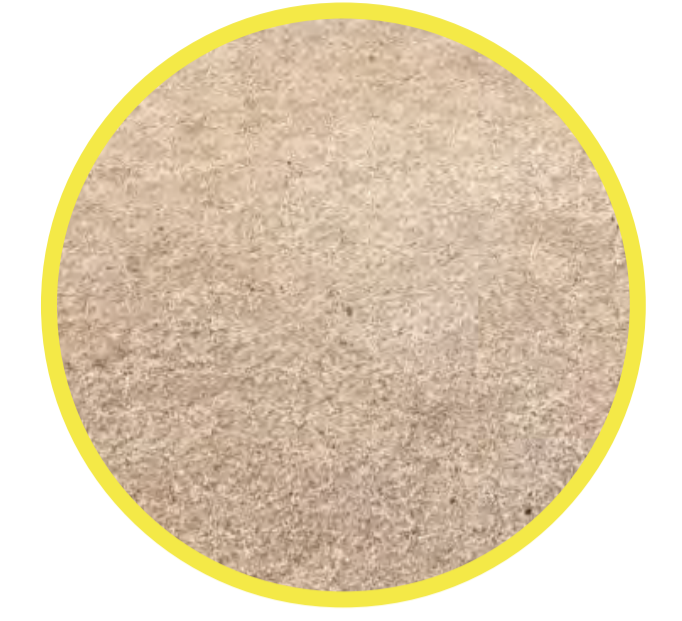
INFORMAL PATHWAY COMPACTED LIMESTONE 5% CONCRETE MIX
